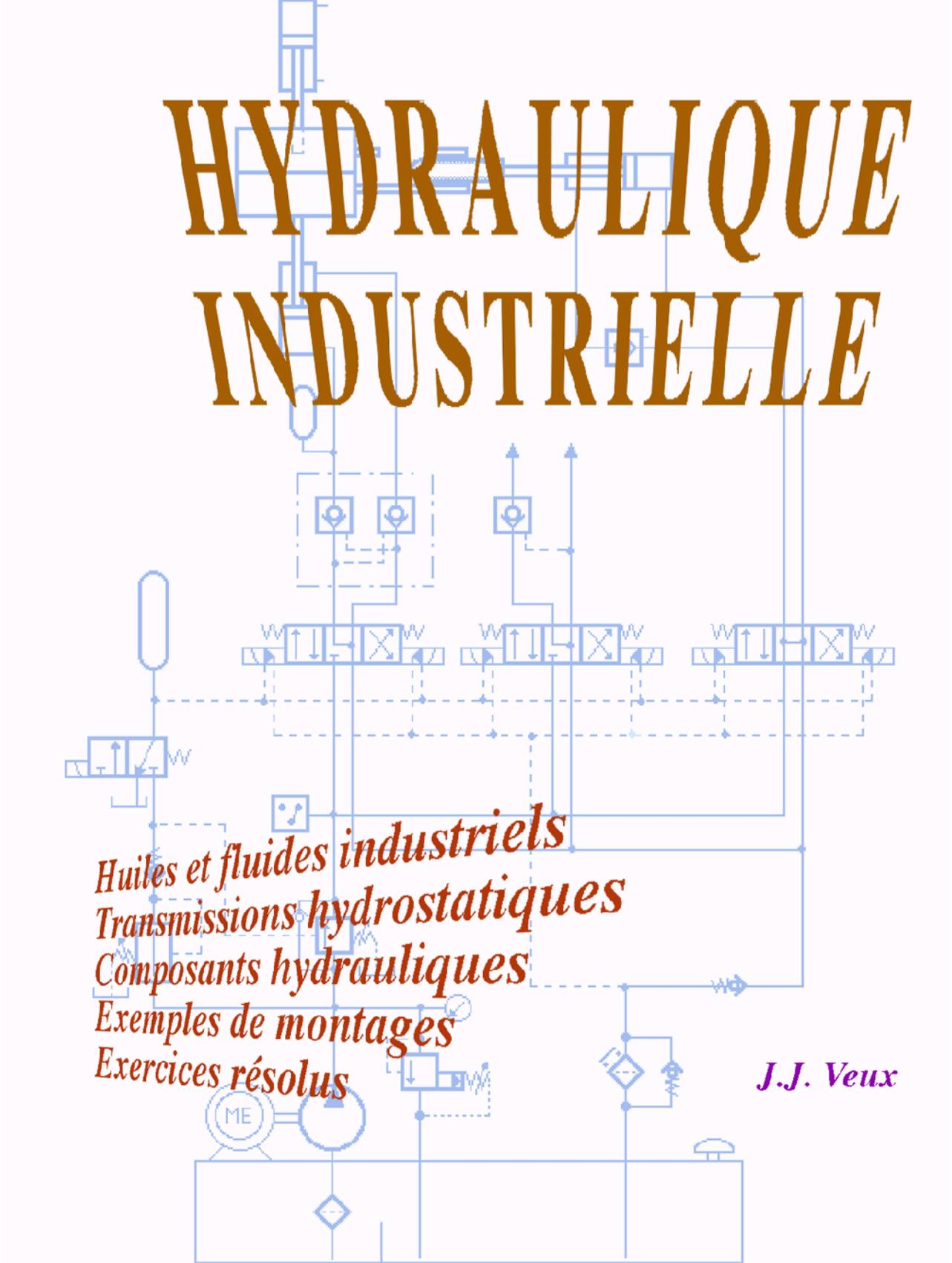
A detailed hydraulic circuit diagram in blue lines serves as the background. It features a pump at the bottom left, a reservoir at the bottom, and a complex network of pipes, valves, and actuators. Three 4/3-way directional control valves are prominently displayed in the middle section. The diagram includes various symbols for pumps, tanks, valves, and actuators, connected by solid and dashed lines representing hydraulic lines.
