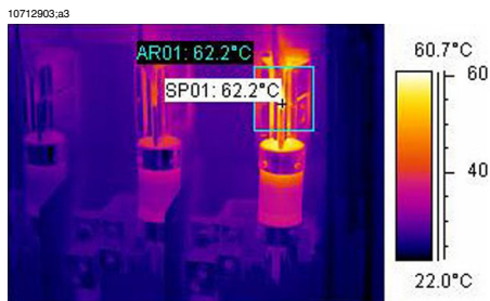
Figure 7.3 An infrared image of a fusebox where the maximum temperature is displayed
